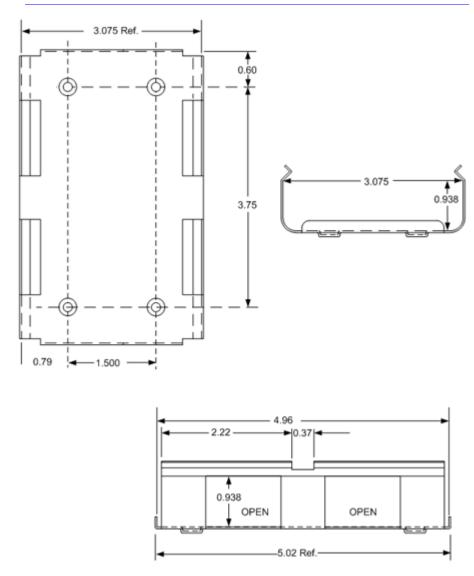
FIGURE 1. Raven Mounting Bracket, part number 100-170-1009 A
